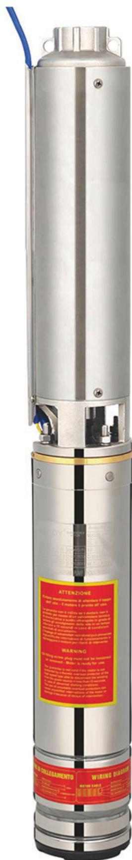
This Slimline submersible borehole pump is suitable for 4" or larger boreholes, wells or reservoirs. Manufactured from corrosion & abrasion resistant materials. This range is manufactured to NEMA standard for submersible motors. Designed for flow rates up to 1.5m<sup>3</sup>/h and heads of up to 325 meters.
